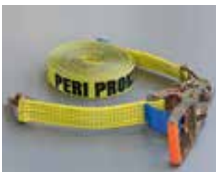
The Tension Belt PTB 12 is tensioned between two supports and forms the sub-construction for the Fold Mesh PFR. The two-piece belt with a length of 12.00 m is equipped with hooks and securing straps.
