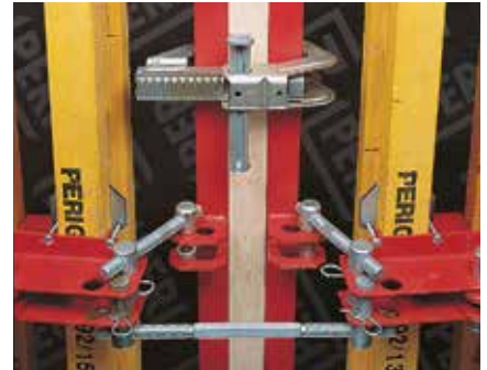
The BFD Alignment Coupler connects the panels; the Adjusting Spindle is only required when the element units are moved.
