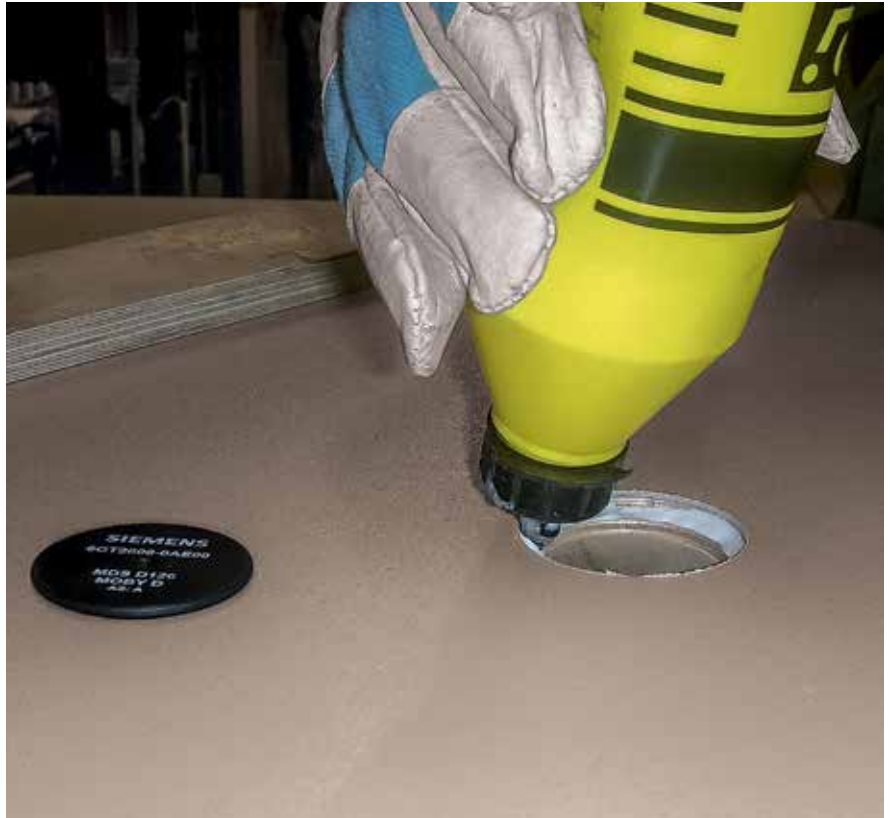
The installation of RFID chips in the PERI Pave production pallets can also be done later using the repair kit.
