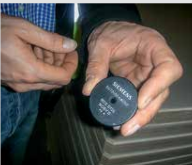
RFID tags for installation in the production pallets: the tags have a permanent unique number which can be used for clear identification of the pallet.
